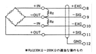
The resister to be used (RZ) directly influences the zero drift characteristic of the sensor, therefore use the resister that has an excellent temperature coefficient. (25ppm/ or less recommended) This method can be used for sensitivity calibration when the indicator is replaced.
